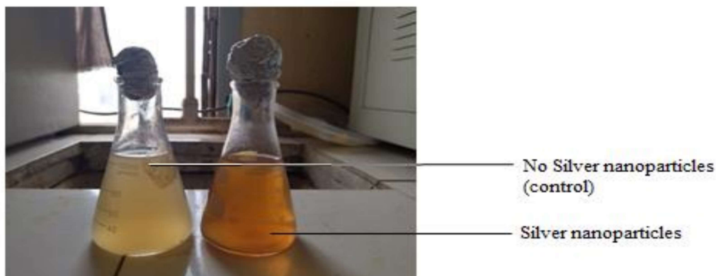
Fig 3: Colour change of the filtrate containing Aspergillus flavus (and AgNO 3 ) to brown
