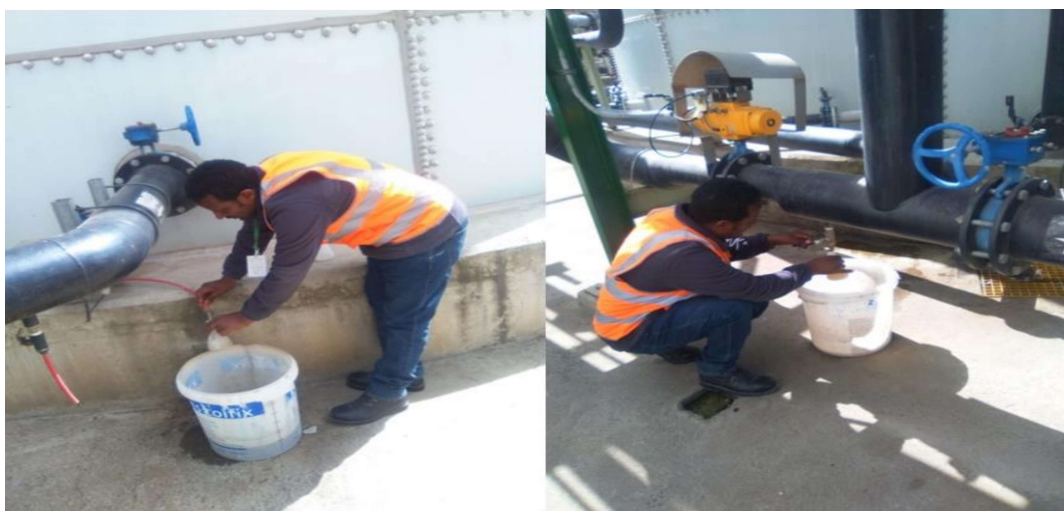
Figure 2. Wastewater Sample collection from the outlet of treatment plants
